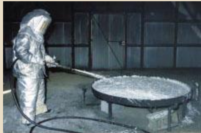
Fire testing in AFFF in a confined space.
