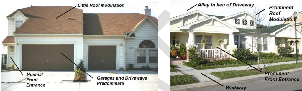
Auto Versus Human Design: Providing rear alleys or side loaded garages enables the home to present itself to the street, which promotes sociability and walkability.
