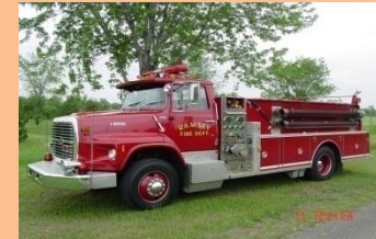
Tanker 21 1989 Ford L9000 750 GPM Pump 1850 Gallons of water Crew of 3
