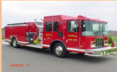
Engine 11 2001 HME 1500 GPM Pump 1000 gallons of water Crew of 6
