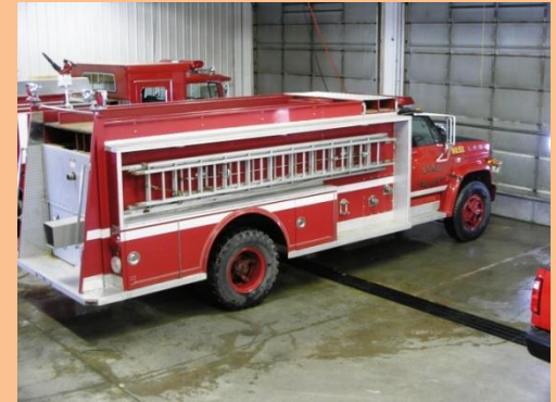
Tanker 31 1986 GMAC 1900 Gallons of water Crew of 3
