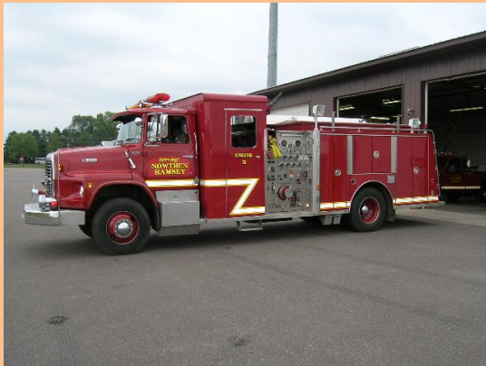
Engine 31 1989 Ford L9000 1250 GPM Pump 1000 gallons of water Crew of 6
