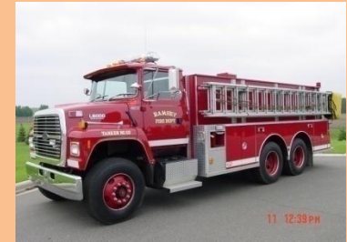
Tanker 11 1990 Ford L9000 3000 gallons of water Crew of 2
