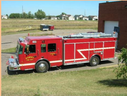
Engine 21 2007 Spartan 1250 GPM Pump 1000 gallons of water Crew of 6
