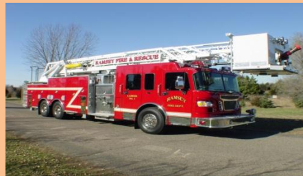
Aerial 21 2003 Spartan 104 Ft Platform 1500 GPM Pump 300 Gallons of water Crew of 6
