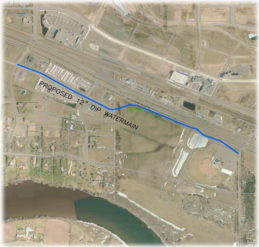
Figure 4. Proposed Water Main improvements.
