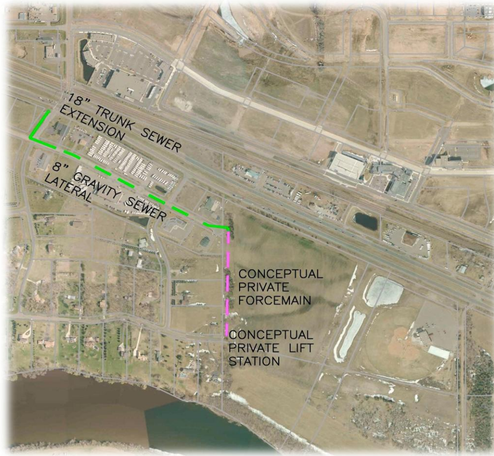
Figure 7. Proposed Sanitary Sewer improvements.
