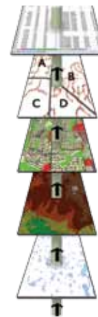
Land use management planning involves a sequence of steps including identifying constraint layers, consolidating layers and creating the core database.
