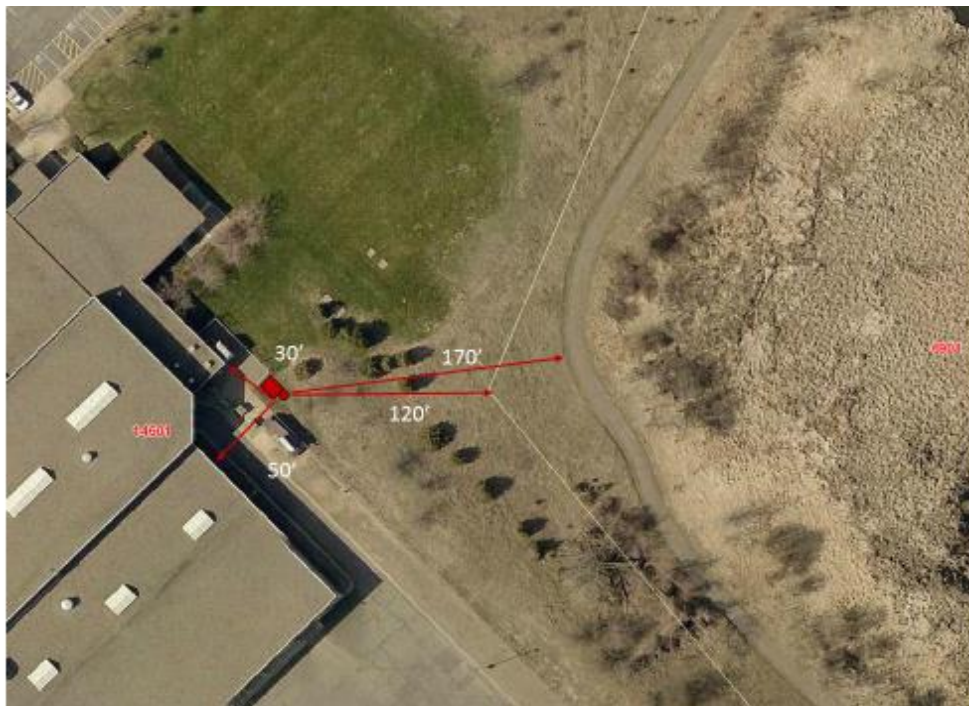
Exhibit 3: Placement of tower on Eastern side of building
