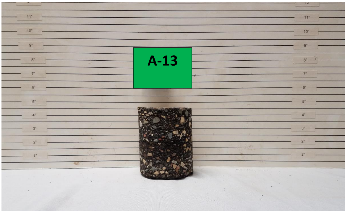
Bituminous Pavement Cores, A-13: 4 ¾ Inches.
