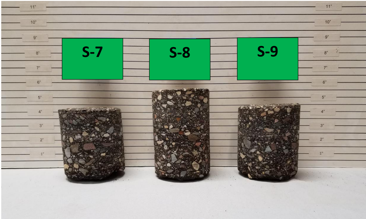
Bituminous Pavement Cores, S-7: 4 ¼ Inches, S-8: 5 ¾ Inches, S-9: 4 ½ Inches.
