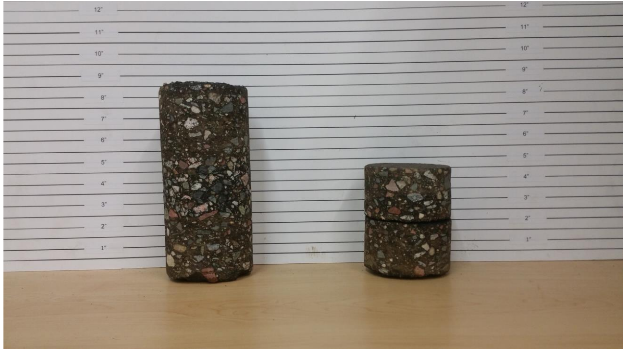
Bituminous Pavement Cores, C-1: 8 ¾ Inches, C-2: 4 ¾ Inches
