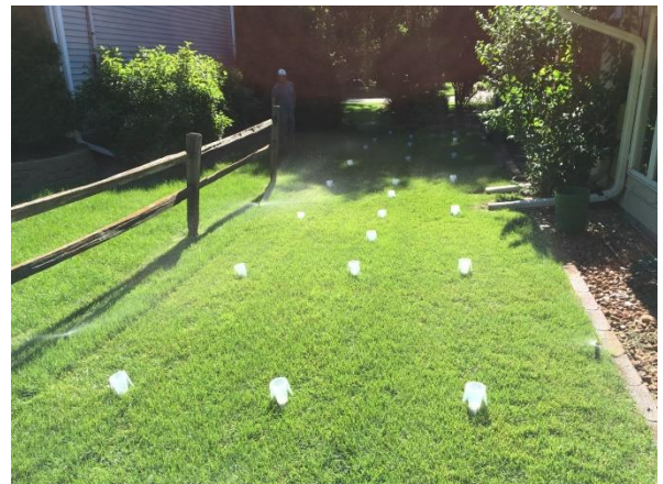
PLACE CATCH CANS ON A GRID PATTERN
