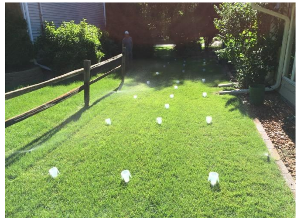
PLACE CATCH CANS ON A GRID PATTERN
