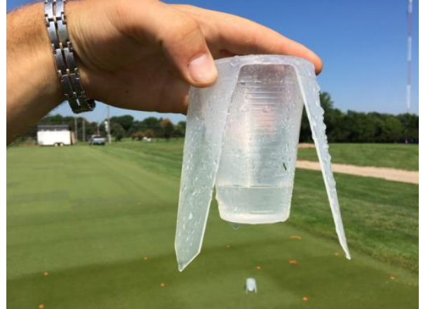
MEASURE THE DEPTH OF WATER IN EACH CAN
