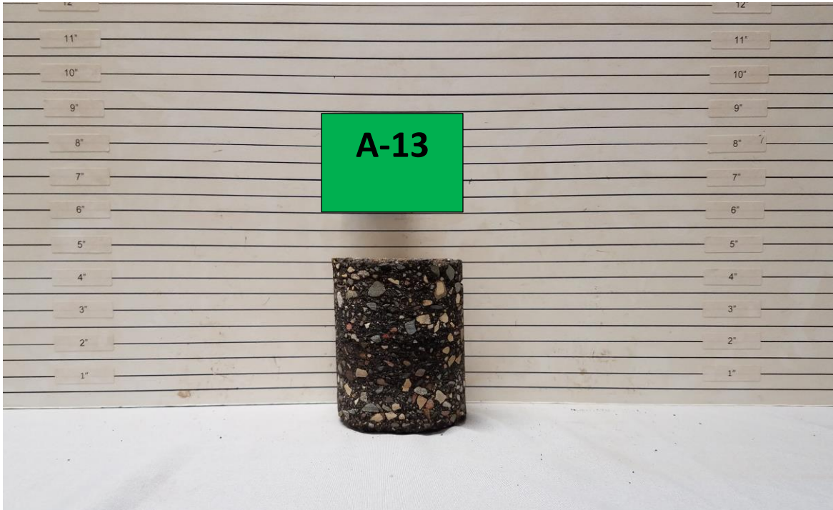
Bituminous Pavement Cores, A-13: 4 ¾ Inches.
