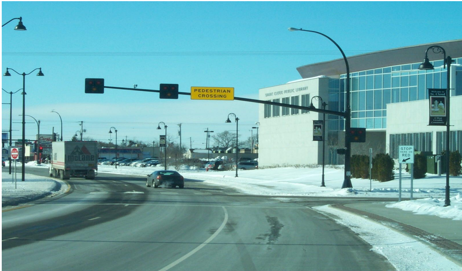
HAWK Beacon at 12 th Ave in St. Cloud WB
