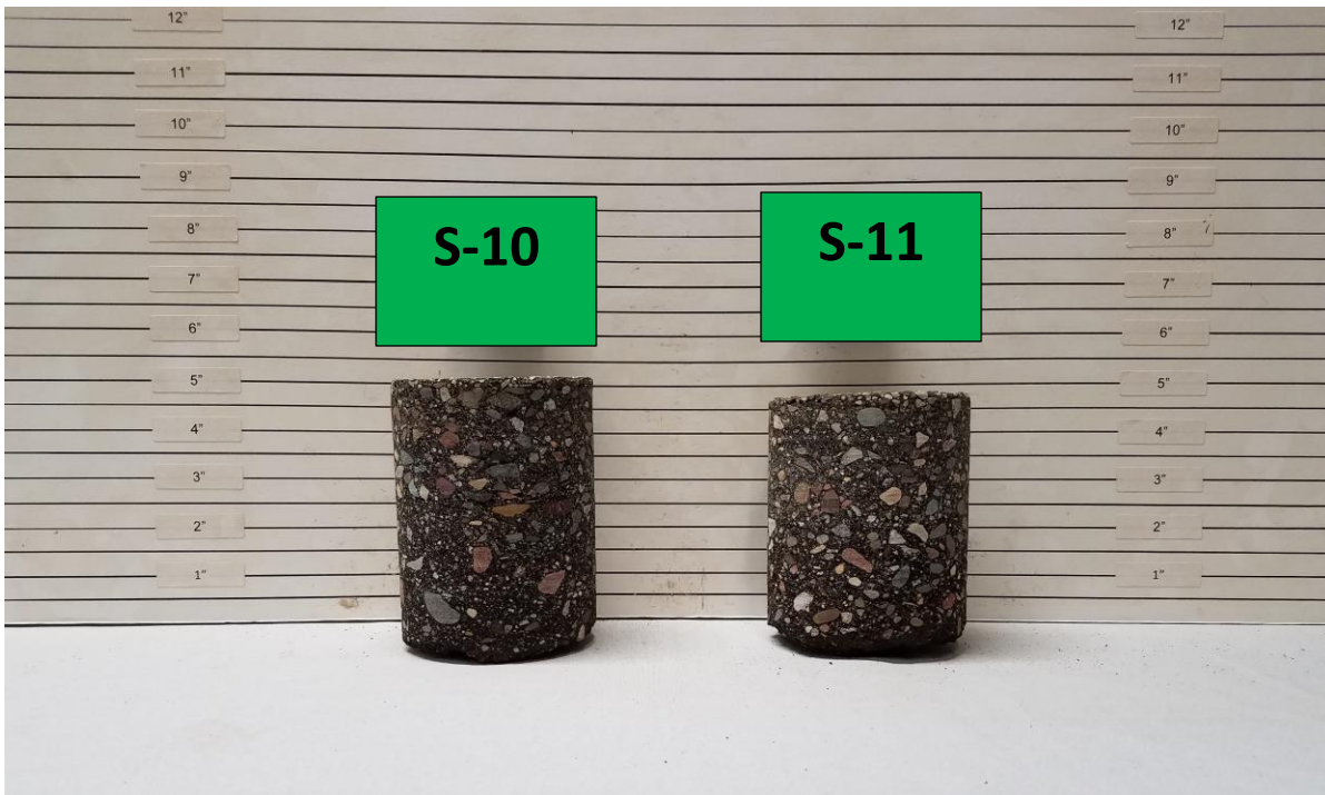
Bituminous Pavement Cores, S-10: 5 Inches, S-11: 4 ¾ Inches.
