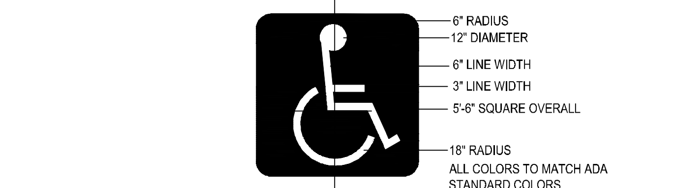
4 ACCESSIBLE PARKING PAVEMENT MARKING NTS
