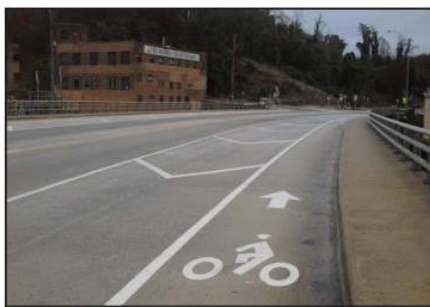
Buffered Bicycle Lane Source: www.pedbikeimages.org / Lyubov Zuyeva
