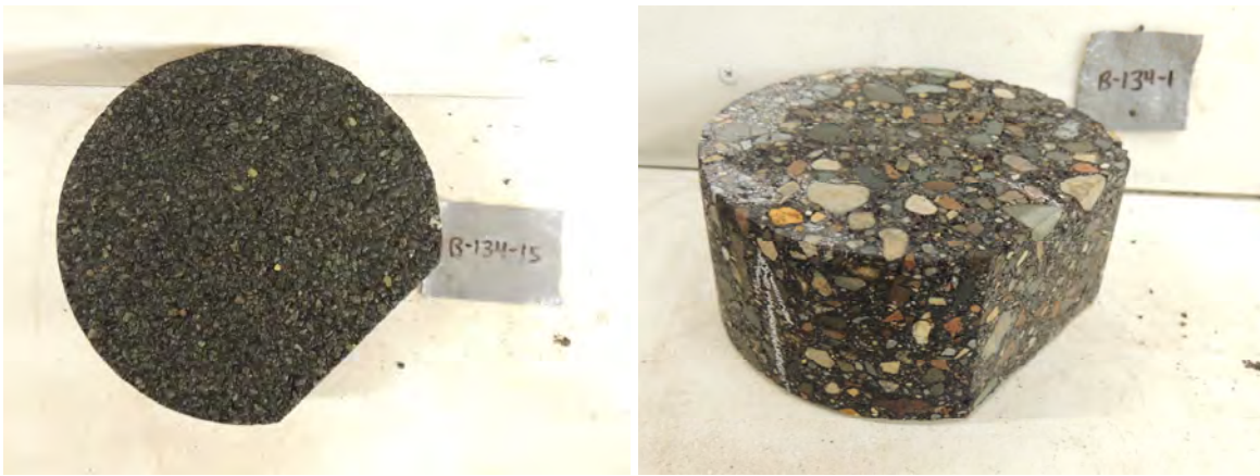
Figure J-5. Paired specimens from 134th Avenue in Burnsville, MN, before Hamburg test
