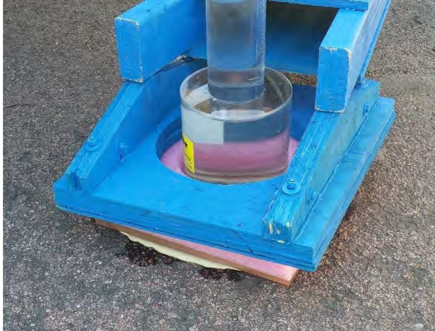
Figure 4. Configuration of the NCAT Permeameter in attempts at field permeability testing
