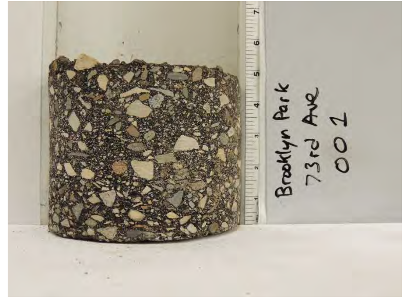
Figure I-3. Coring operations and sample core extracted from 73rd Avenue in Brooklyn Park, MN
