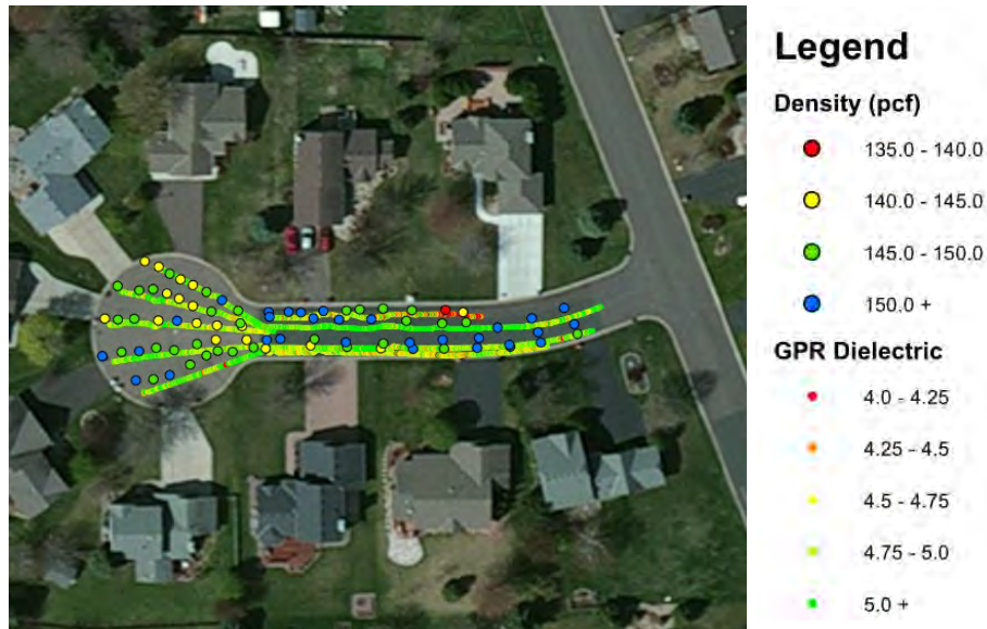
Figure 10. Map of dielectric and density data collected at Newbury Alcove site in Woodbury, MN
