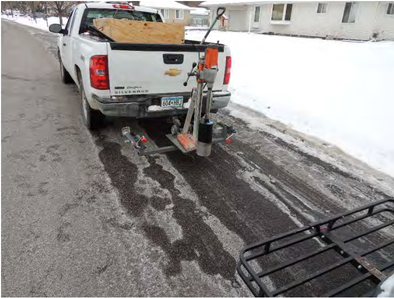
Figure I-9. Coring operations and sample core extracted from Hyde Ave in Cottage Grove, MN
