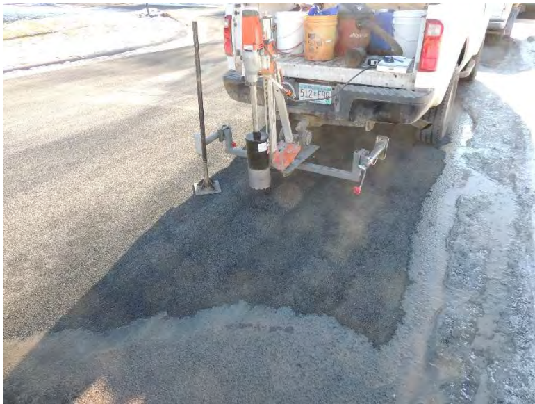
Figure I-4. Coring operations and sample core extracted from Louisiana Avenue in Brooklyn Park
