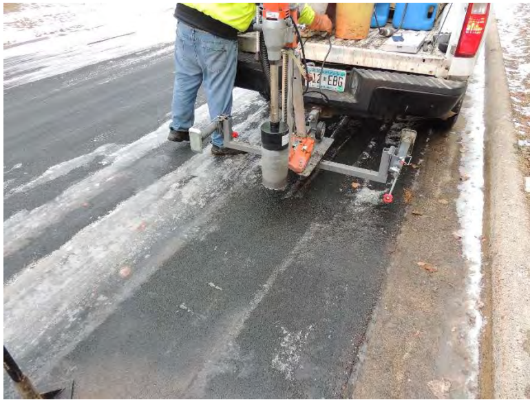
Figure I-13. Coring operations and sample core extracted from Osseo, MN
