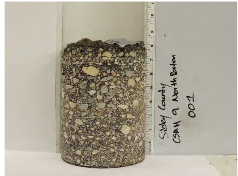
Figure I-14. Coring operations and sample core extracted from the north part of CSAH 9 in Sibley County, MN
