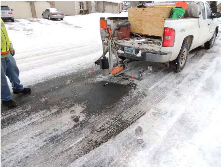
Figure I-16. Coring operations and sample core extracted from Bridgewater Road in Woodbury, MN
