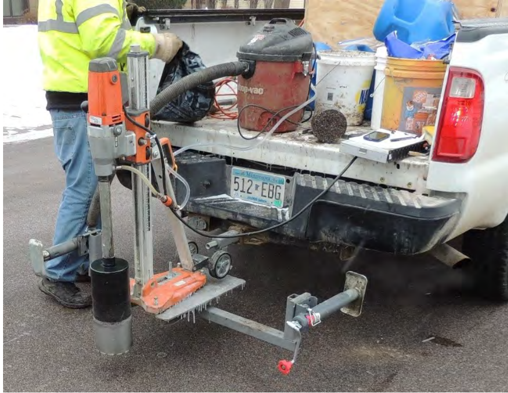
Figure 3. Truck-mounted rig used to obtain cores on-site
