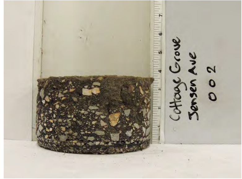
Figure I-11. Coring operations and sample core extracted from Jensen Ave in Cottage Grove, MN
