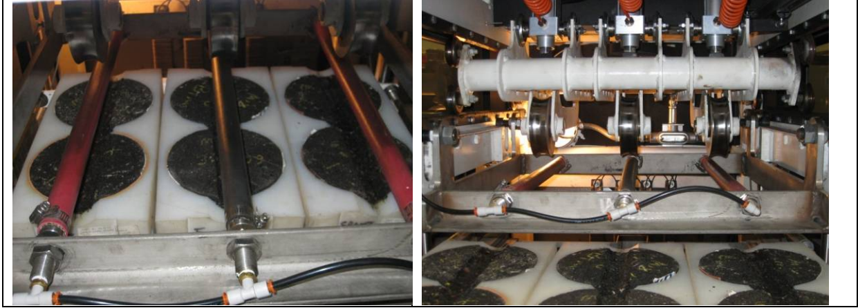
Figure 2.8. Asphalt Pavement Analyzer (APA), or Rut Tester
