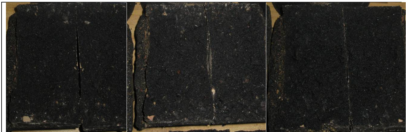
Figure 2.11. Visual Examination of APA ‘wet’ specimens
