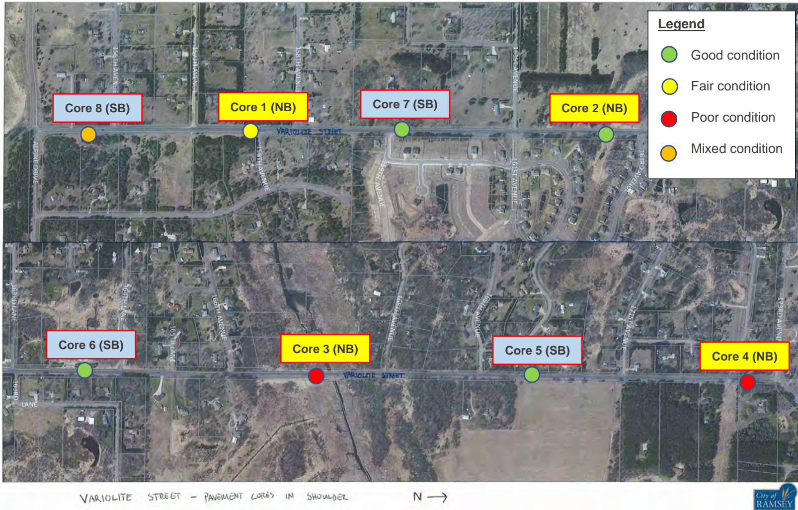
Figure 1. Pavement core locations along the shoulder of Variolite Street.
