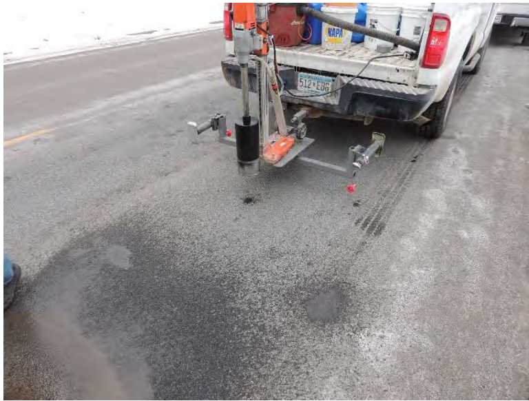
Figure I-5. Coring operations and sample core extracted from Winnetka Avenue in Brooklyn Park, MN
