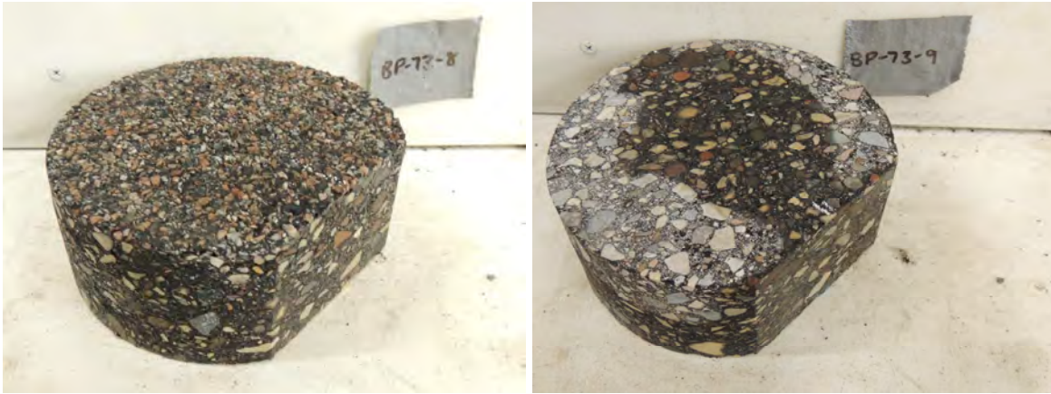
Figure J-3. Specimen from 73rd Avenue in Brooklyn Park, MN, after Hamburg test
