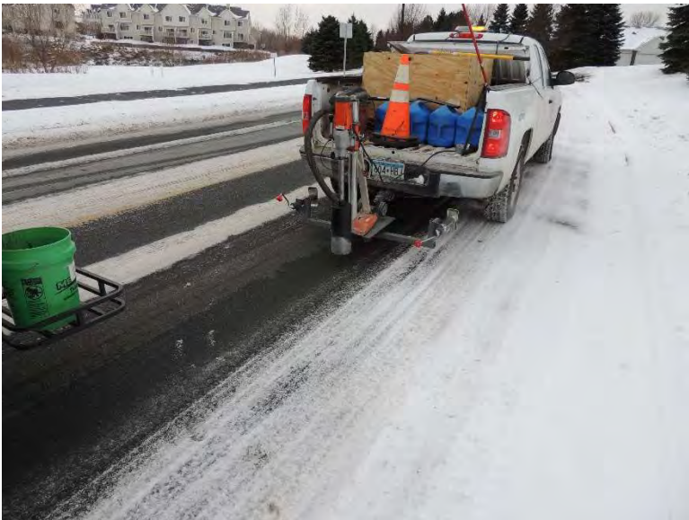
Figure I-12. Coring operations and sample core extracted from Brooks Blvd. in Inver Grove Heights, MN
