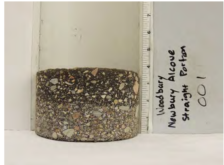
Figure I-18. Coring operations and sample core extracted from Newbury Alcove straight portion in Woodbury, MN
