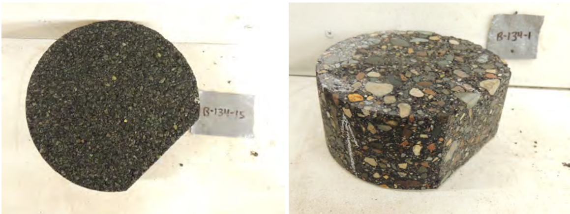
Figure J-5. Paired specimens from 134th Avenue in Burnsville, MN, before Hamburg test
