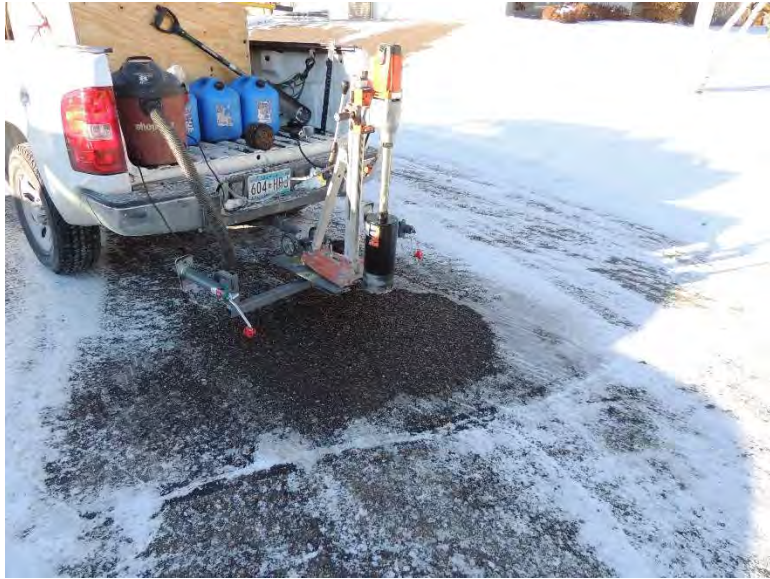
Figure I-17. Coring operations and sample core extracted from Newbury Alcove Cul de sac in Woodbury, MN
