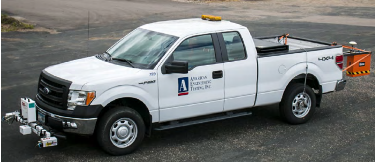
Figure 5. Vehicle-mounted GPR used for site evaluation
