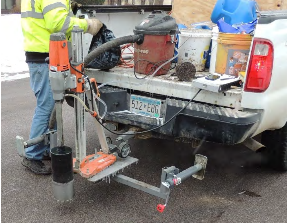
Figure 3. Truck-mounted rig used to obtain cores on-site
