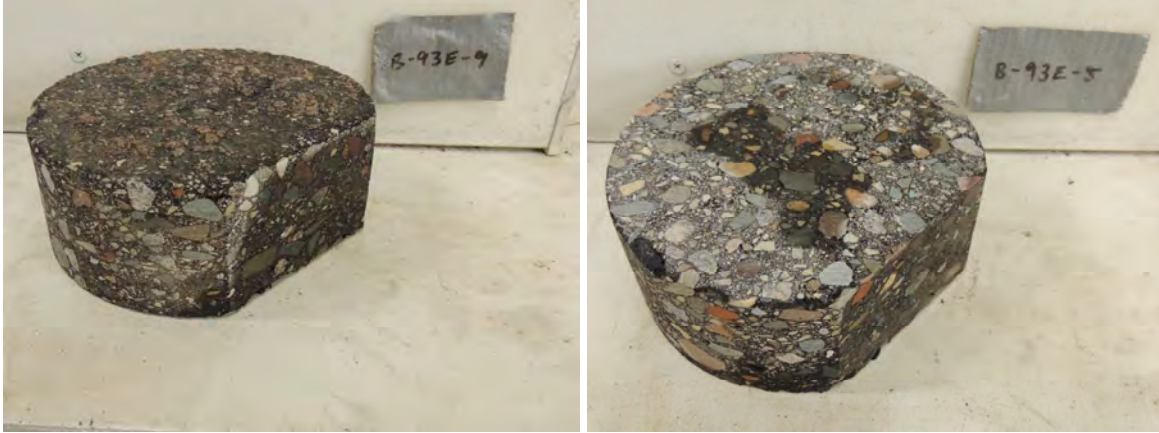
Figure J-1. Paired specimen from the east end of 93rd Avenue in Blaine, MN, before Hamburg test
