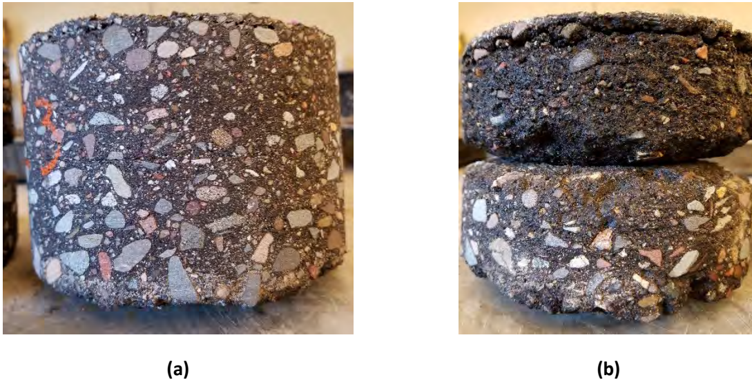
Figure 9. (a) Intact core and (b) core stripped under chip seal and between asphalt lifts, recovered from city of Shoreview, MN
