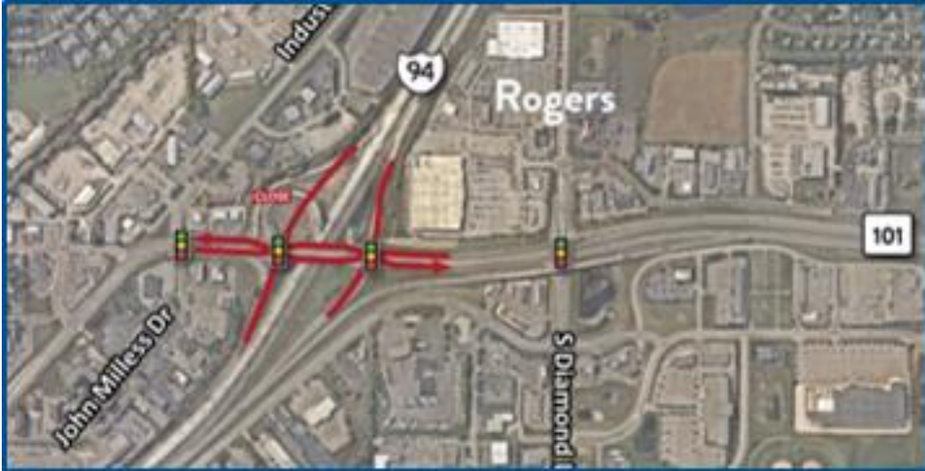
Figure 37: I-94/Hwy 101 Interchange – Condition 1 (DDI)
