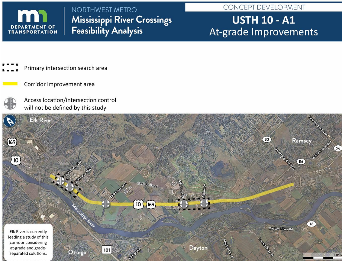
Figure 17: Highway 10-A1: At-Grade Improvements
