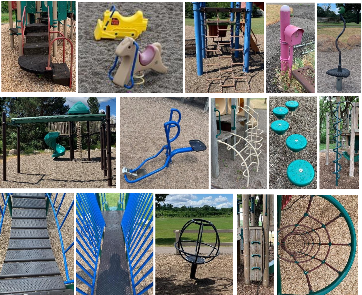
Figures 5-19: Playground Equipment: (left to right, top to bottom) transfer surface; spring rider; chain ladder; talk tube; spinner; track-ride; sandbox excavator toy; metal ladders; stepping pods; corkscrew climber; clatter bridge; belt bridge; globe spinner; climbing wall with rope; enclosed rope climber.
