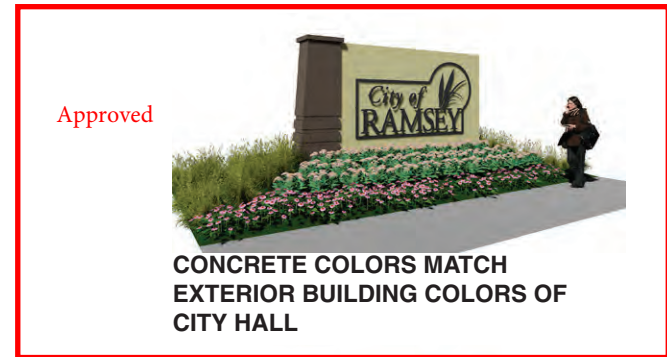
LIGHT COLORED CONCRETE WITH METAL PANEL CUT-OUT LETTERING
