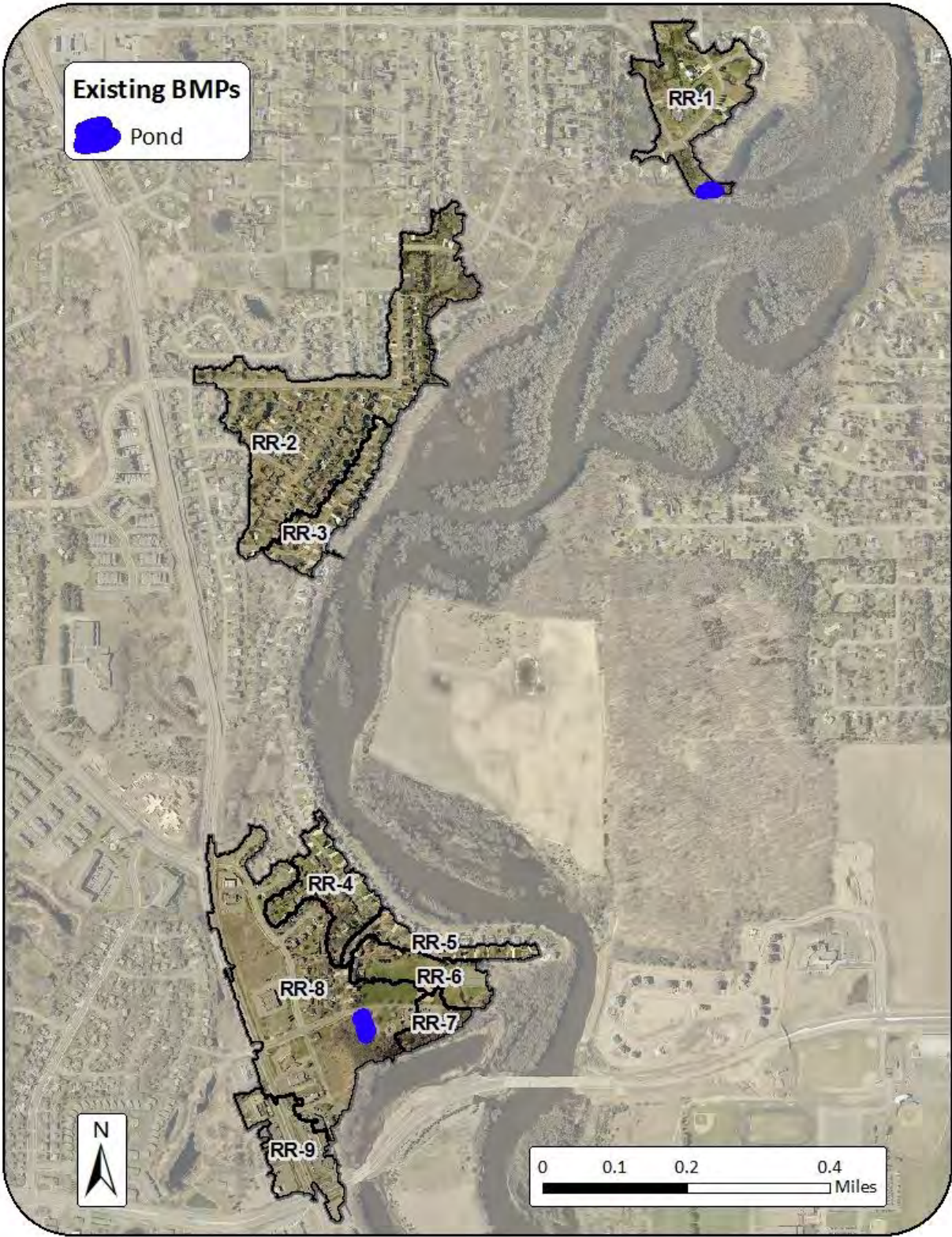
Figure 2: Rum River network-wide map showing existing BMPs included in the WinSLAMM model. Street sweeping is not shown on the map but was included where applicable in catchments within the network.
