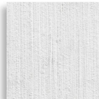
Light Broom Finished TILT-UP CONCRETE EXAMPLE
