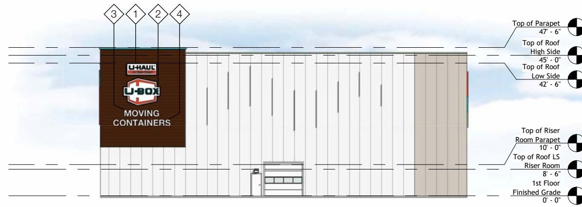
NORTH ELEVATION - BLDG. B
