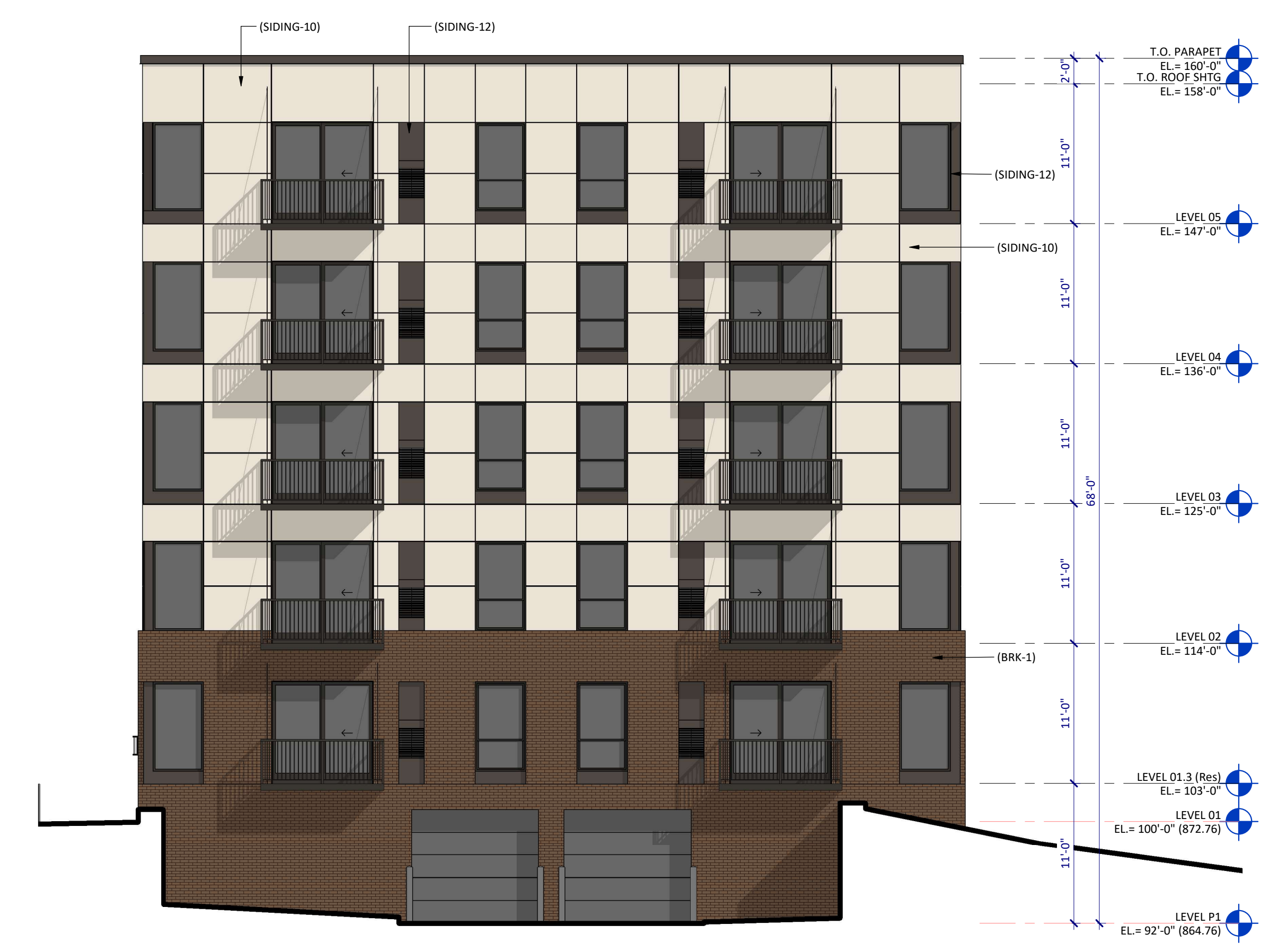
4C EXTERIOR ELEVATION - EAST - AREA B SCALE: 3/8" = 1'-0"
