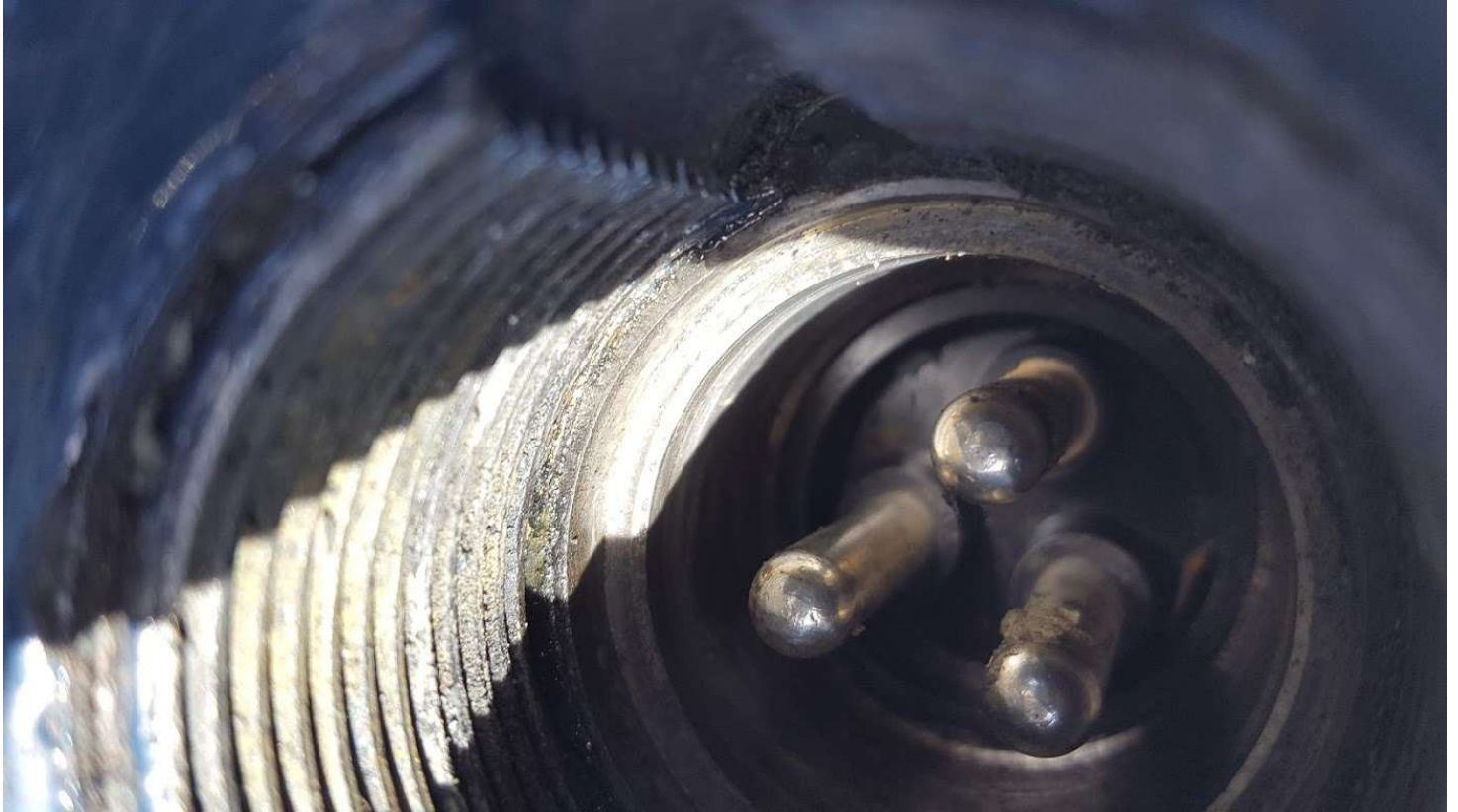
Figure 2.2.5- View of the internal components of the connector. Note: Once the cable was removed, the resistance remained low as throughout the previous measurements, pointing to internal components of the motor.
