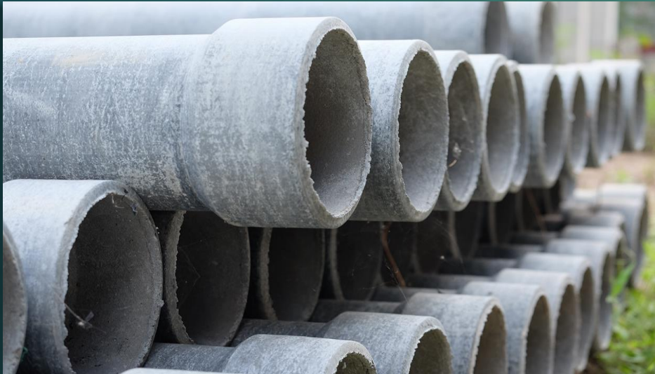
▶ Asbestos-Cement (AC) Pipe
