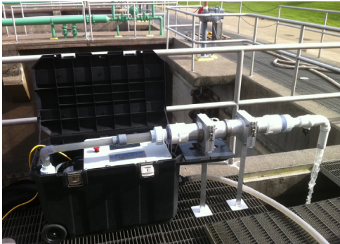
Hammerhead on-site screen sizing test to determine the proper design and size
