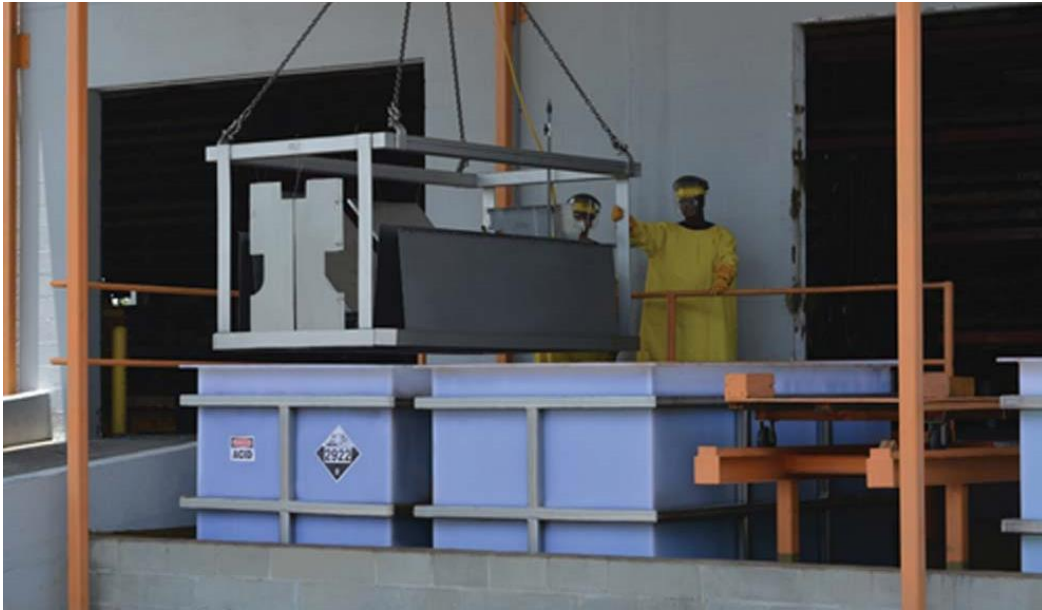
Pickling and Passivation Process – Clearwater Facility
