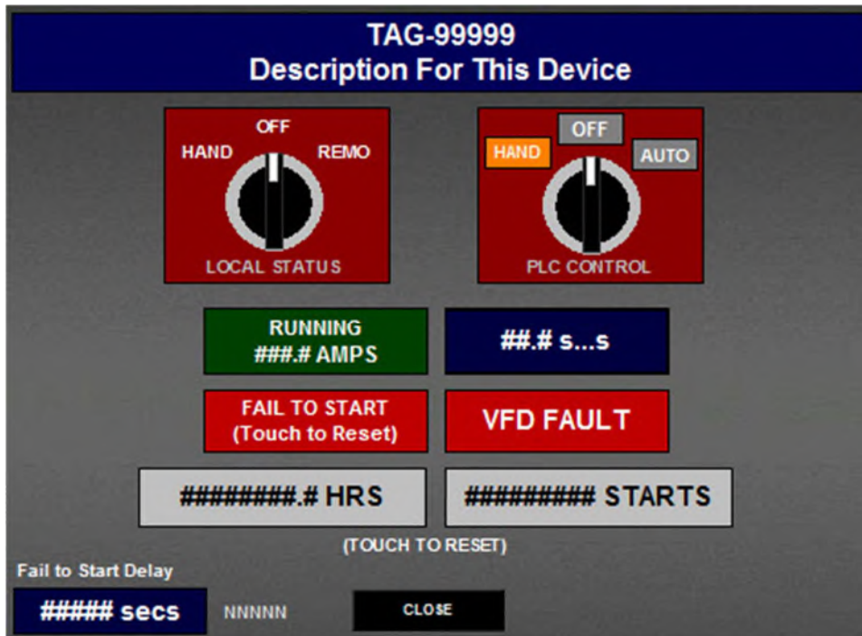
Figure CP – 8 : Equipment Control Pop-Up Screen EXAMPLE ONLY. Actual screens may vary.
