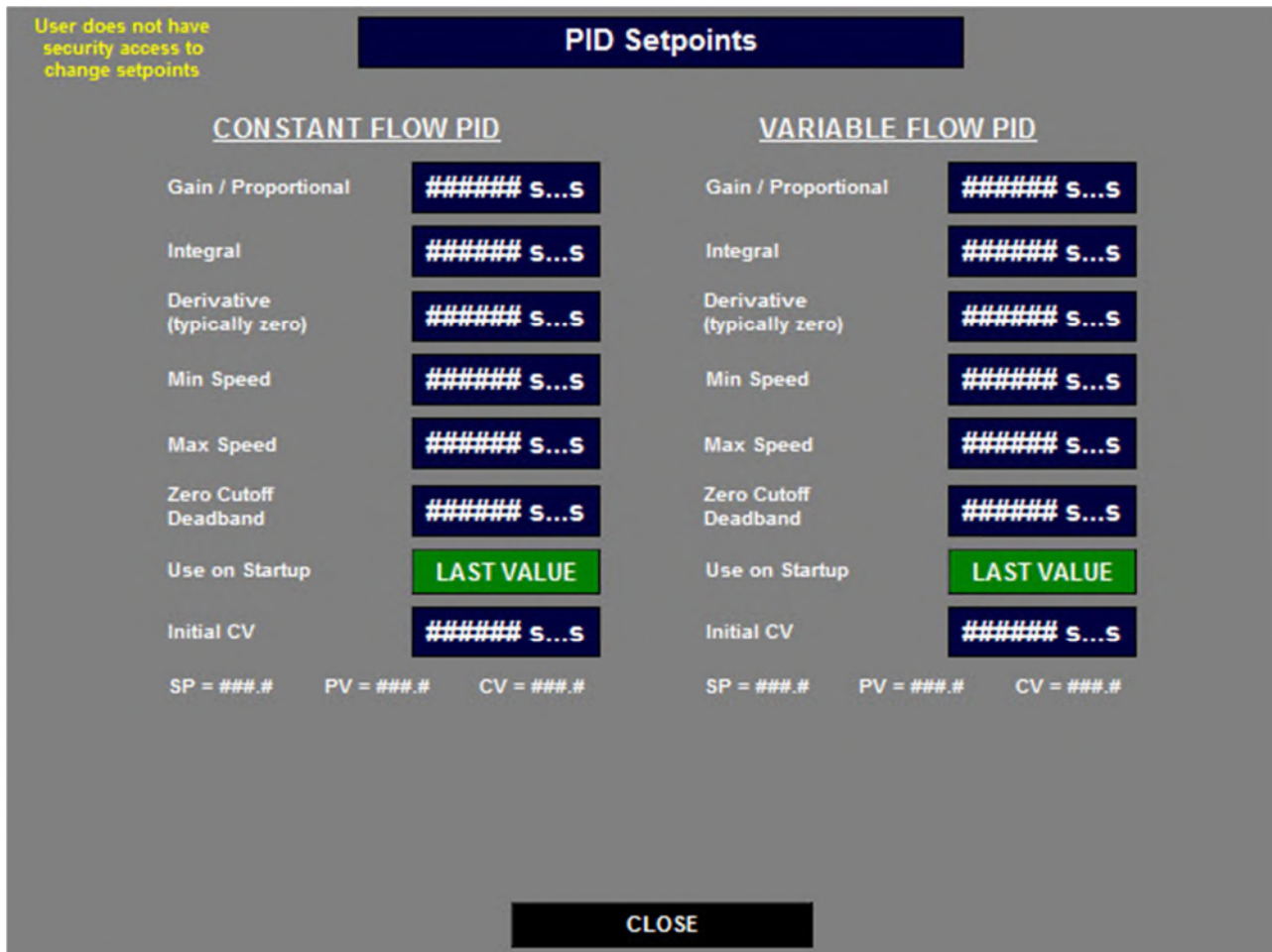
Figure CP-7 : PID Setpoints Screen EXAMPLE ONLY. Actual screens may vary.
