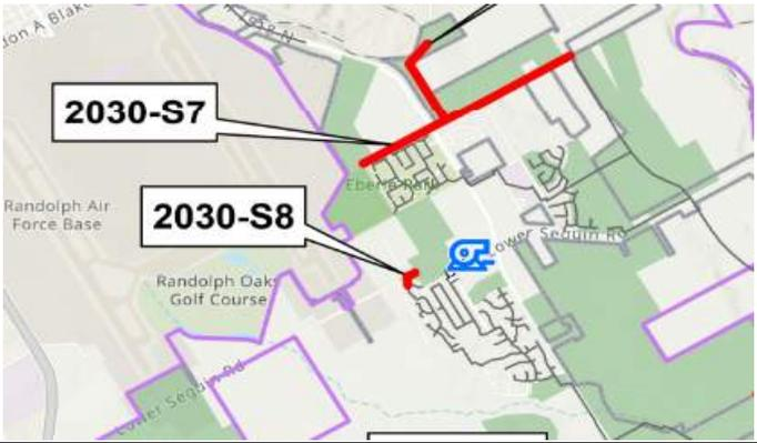
The map displays the project area in a residential neighborhood. A red line indicates the proposed 8-inch gravity line along Aranda. Two callout boxes identify specific project segments: 2030-S7 and 2030-S8. Key landmarks shown include Randolph Air Force Base to the west and Randolph Oaks Golf Course to the south. A blue logo is visible near the project site.
