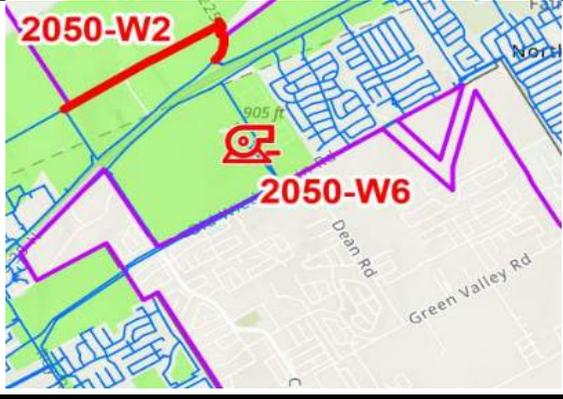
The map displays the project location in a residential area. A red line labeled '2050-W2' indicates a water main connection. A red circle with a pump symbol labeled '2050-W6' marks the location of the 3.0 MG Gravity Storage Tank (GST). The map also shows 'Dean Rd' and 'Green Valley Rd'.
