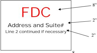
**Sprinkler riser rooms** shall have a sign on the door visible from the exterior of building. The sign shall be mounted directly to the door unobstructed, have RED reflective letters on a WHITE background or WHITE reflective letters on a RED background and be made of a durable material. Doors may be painted or stenciled, Sign shall be 24" X 24" (inches) and have 8" (inch) lettering. Group R occupancies may have smaller signs if approved by Fire Marshal's Office.
