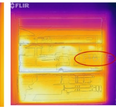
Without WinSert Interior surface temperature 116.7°
