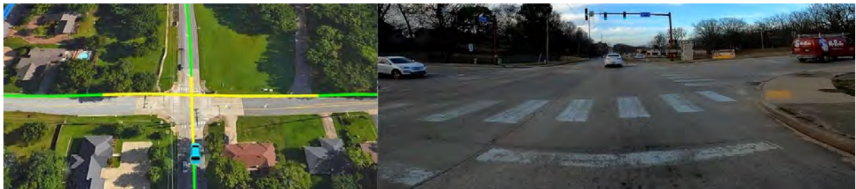
Figure 11 - Geolocated Video, Stripe in FAIR Condition
