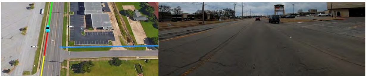
Figure 12 - Geolocated Video, Stripe in LOST Condition
