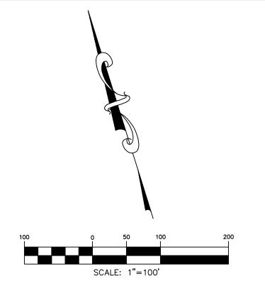
THE BEARINGS SHOWN HEREON ARE ORIENTED TO THE TEXAS STATE PLANE COORDINATE SYSTEM, CENTRAL ZONE, NAD 83, 93 ADJUSTMENT.
