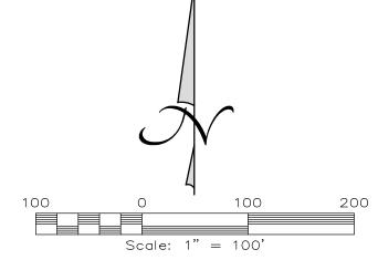
BEARINGS CITED HEREON BASED ON STATE PLANE COORDINATES, GRID NORTH, CENTRAL ZONE, TEXAS NAD 83 (93).
