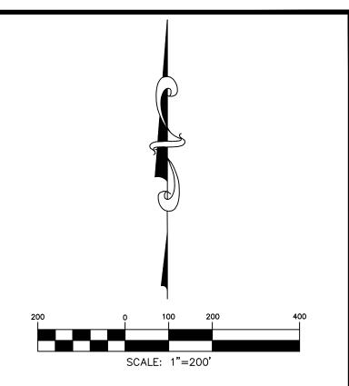
THE BEARINGS SHOWN HEREON ARE ORIENTED TO THE TEXAS STATE PLANE COORDINATE SYSTEM, CENTRAL ZONE, NAD 83, 93 ADJUSTMENT. DISTANCES ARE EXPRESSED AS GRID VALUES. TO CONVERT TO SURFACE VALUES, DIVIDE BY THE COMBINED SCALE FACTOR OF 0.999921534411
