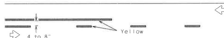
REFLECTORIZED PAVEMENT MARKINGS - PATTERN B
