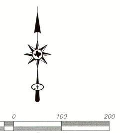
Bearings and coordinates shown hereon based on Texas State Plane Coordinate System Central Zone (NAD83). Distances shown hereon are surface distances. Combined Scale Factor = 0.99984640
