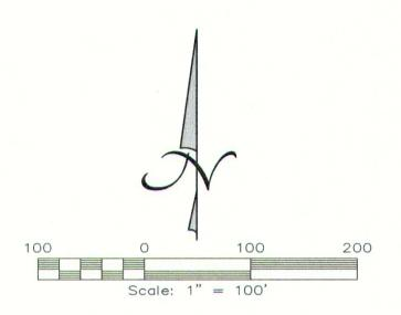
BEARINGS CITED HEREON BASED ON STATE PLANE COORDINATES, GRID NORTH, CENTRAL ZONE, TEXAS NAD 83 (93).
