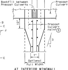
AT INTERIOR WINGWALL (Precast Culvert)
