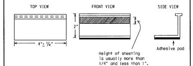
STAPLES OR NAILS SHALL NOT BE USED TO SECURE TEMPORARY FLEXIBLE-REFLECTIVE ROADWAY MARKER TABS TO THE PAVEMENT SURFACE
