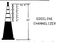
1. This device is intended only for use in place of a vertical panel to channelize traffic by indicating the edge of the travel lane. It is not intended to be used in transitions or tapers.
