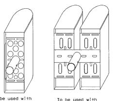
To be used with 2½" OD RR or thinwall Steel posts. To be used with thinwall Steel posts. Not to be used with RR posts.
