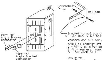
— Bracket to mailbox attachment: 6 - ¼" Dia, x ¾" bolt w/ 2 flat washers and nut per each bolt. Angle to bracket attachment: 2 -  $\frac{1}{3}$ " Dia. x  $\frac{3}{4}$ " bolt with 2 flat washers, lock washer and nut per each bolt. Angle to
