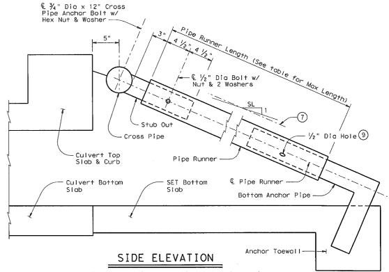
(Showing Pipe Runner with Cross Pipe Connection option A1 and anchor Pipe option B2. Wingwall not shown for clarity)
