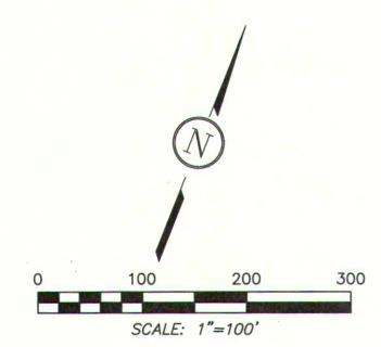
BEARING BASIS: THE TEXAS COORDINATE SYSTEM OF 1983 (NAD83) CENTRAL ZONE. DISTANCES ARE SURFACE. SURFACE TO GRID COMBINED SCALE FACTOR 0.9998800.
