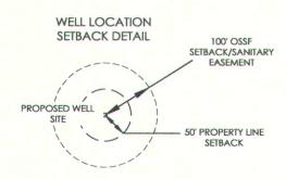
NOTE: THE LOCATIONS SHOWN HEREON ARE FOR CONCEPTUAL PURPOSES ONLY. ALL WELL LOCATIONS MUST BE APPROVED BY THE PROPER AUTHORITY PRIOR TO BEING CONSTRUCTED.
