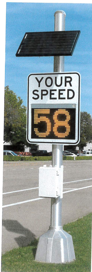
12" model shown with optional YOUR SPEED aluminum MUTCD compliant bezel, solar panel, and battery system
