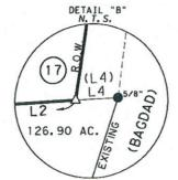
NO. DIRECTION DISTANCE L1 N73° 05′ 59"E 73.18' L2 S66° 59' 08"W 105.21' L3 N73° 05′ 59" E 5.98' (L3)(N73° 06′ 08"E) (5.98')L4 N66° 59' 08"E 10.56' (S66° 56′ 31 "W) (L4)(10.56'
