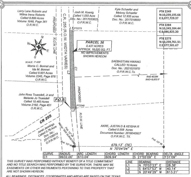
ALL BEARINGS, DISTANCES, COORDINATES AND AREAS ARE BASED ON THE TEXAS COORDINATE SYSTEM OF 1983 (NAD83), TEXAS CENTRAL ZONE, BASED ON GPS SOLUTIONS FROM THE NATIONAL GEO DETIC SURVEY (NGS) ON-LINE POSITIONING USER "PRELIMINARY, THIS SERVICE (OPUS).
