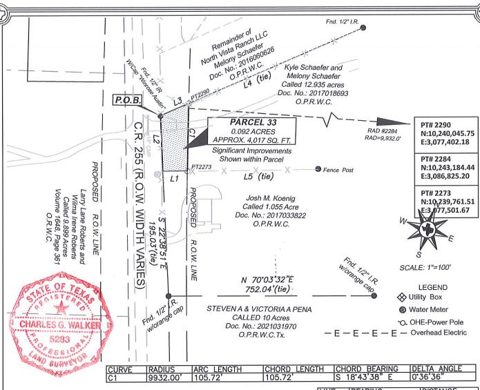
ALL BEARINGS, DISTANCES, COORDINATES AND AREAS ARE BASED ON THE TEXAS COORDINATE SYSTEM OF 1983 (NAD83), TEXAS CENTRAL ZONE, BASED ON GPS SOLUTIONS FROM THE NATIONAL GEO DETIC SURVEY (NGS) ON-LINE POSITIONING USER SERVICE (OPUS).
