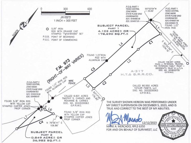
LINE TABLE NUMBER BEARING DISTANCE S 82°24'59" E 210.06 L1 L2 S 07°45'29" W 467.44' L3 N 83°17'06" W 167.22 14 N 07°23'04" F 717.31 L<sub>5</sub> N 86°09'35" E 57.57 L6 N 76°56'41" E 115.38 N 07°17'25" E L7 368.30 L8 N 15°05'09" E 39.94
